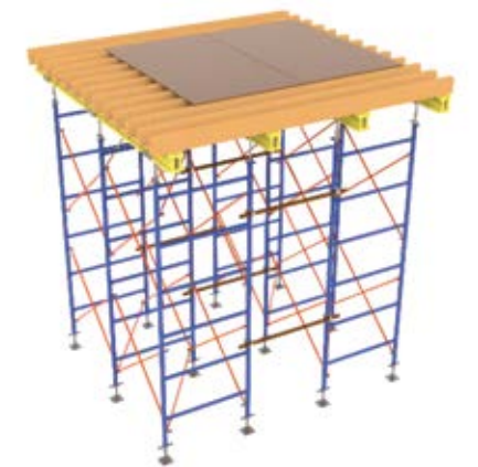
Secondary: Timber Beam Main: H20 Beam
