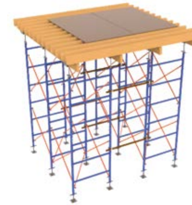
Secondary: Timber Beam Main: Timber Beam
